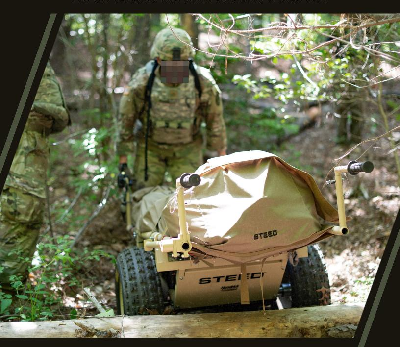
Silent Tactical Energy Enhanced Dismount (STEED) is a lightweight, all-terrain wheeled platform which carries 500 lbs. and has a range of 15-30 miles on one battery pack. The unit is manually operated by a thumb controlled throttle at speeds up to 6.5 mph, in both forward and reverse. It has a zero degree turn radius, is tactically silent, has zero emissions and is completely submersible.
