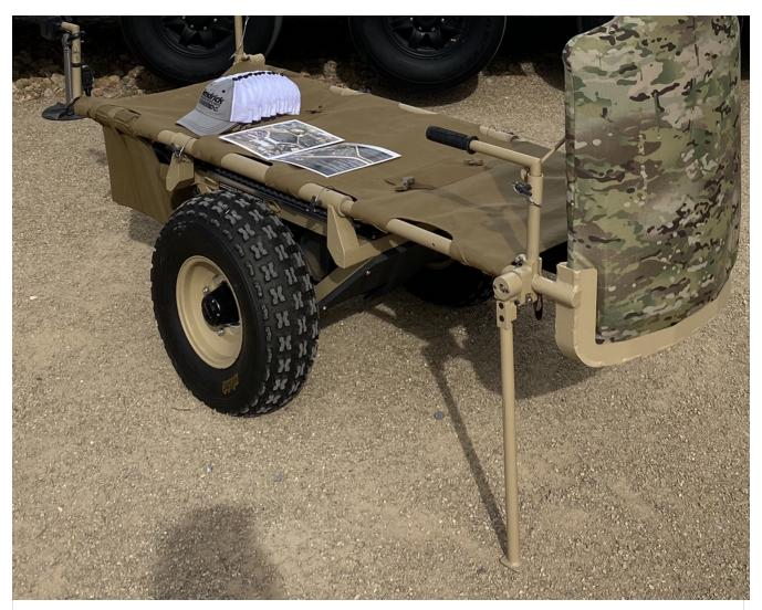
The STEED remains capable of improving mobility and load carriage for the squad. This electric cart has zero emissions and can carry up to 500 lbs over complex terrain at speeds from 0-6.5 mph. STEED will even climb stairs and can be used in water.
